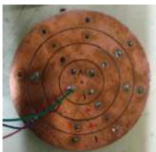
Gambar 8. Susunan LED bagian belakang
